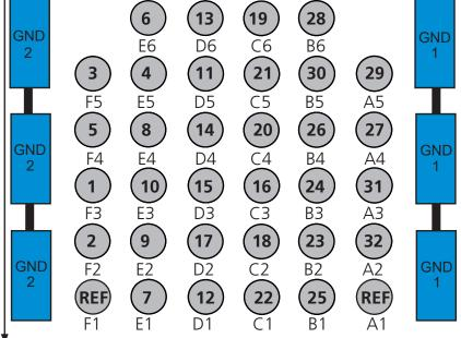
▼ Direction to the connector. The letter digit code below the electrode refers to the position of the electrode in the grid. The numbers inside are the linear channel numbers in Multi Channel Experimenter and MC\_Rack.
