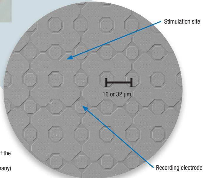
Electron micrograph of the CMOS-chip surface (NMI Reutlingen, Germany)
